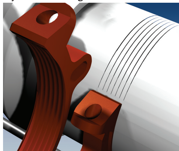
Restraint Ring Tooth Impressions on PVC Pipe.
