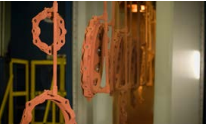
Figure 1.2 Series 2000PV primary casting body exiting powder coat booth
